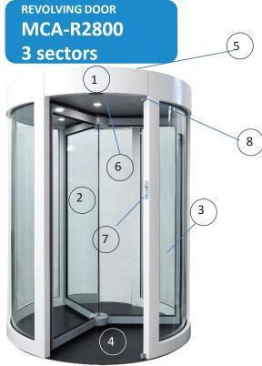
The revolving door MCA-R 2800 is fitted with 3 wings placed at 120° 3 rotating sectors with a passage of 1250 mm in the point of access to the sector and with an overall diameter of the structure of 2800 mm.
