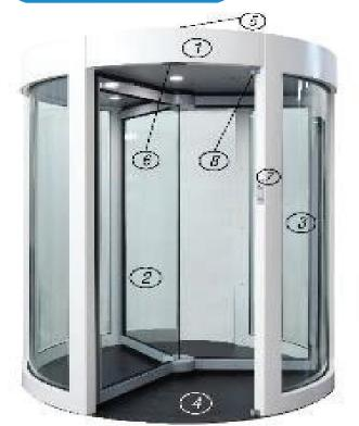
The product MCA-R3800 is fitted with 3 wings at 120° creating 3 rotating sectors with a passage of **1750 mm** in the point of access to the sector and with an overall diameter of the structure of **3800 mm**.
