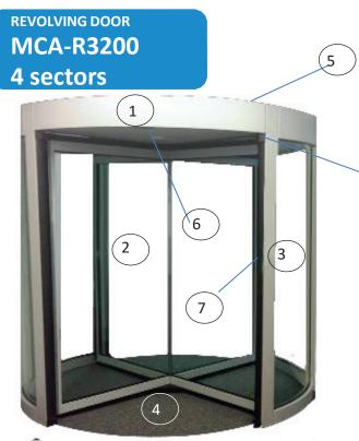
The product MCA-R3200 is fitted with 4 wings at 90° creating 4 rotating sectors with a passage of **2100 mm** in the point of access to the sector and with an overall diameter of the structure of **3200 mm**.
