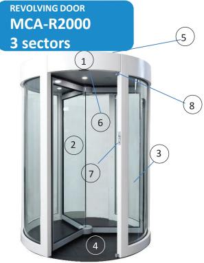
The revolving door MCA-R 2000 is fitted with 3 wings placed at 120° 3 rotating sectors with a passage of 900 mm in the point of access to the sector and with an overall diameter of the structure of 2120 mm.
