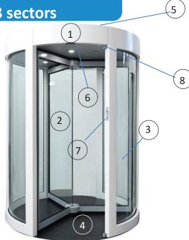
The revolving door MCA-R 2300 is fitted with 3 wings placed at 120°3 rotating sectors with a passage of 1000 mm in the point of access to the sector and with an overall diameter of the structure of 2300 mm.
