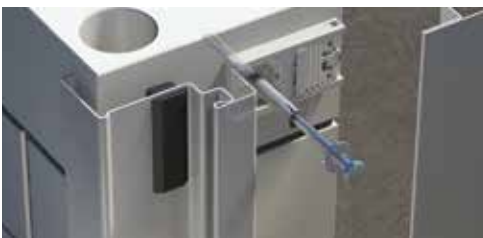
Concealed installation of the counter frame with special fold anchor
