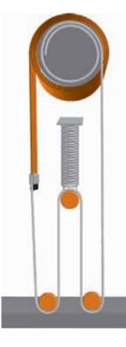
The EFAFLEX wind load system provides permanent door leaf tension. Perfect where wind or negative pressure causes a draft!
