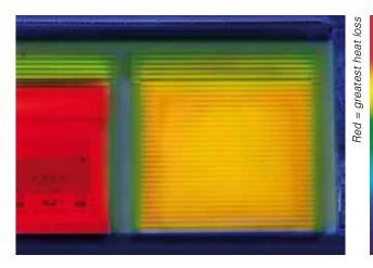
This thermal image of a conventional roller door clearly shows the loss of heat to the outside.
