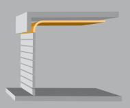
The low header model is used for example in underground parking and car parks.
