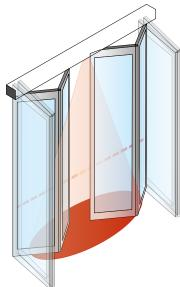
Motion detectors offer a contactless entrance. Further control elements as push-buttons, pull switches or contact carpets can be connected according to the situation. By means of the program switch Bedis you can select the door functions "Manual-Automatic-Open-Night-Exit". Light barriers / scanning safety beam and auto-reverse mechanism make sure one can enter safely.
