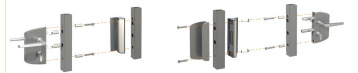
Standardisation of a gate wing. The lock, keep and the counter pullbox are all installed in the same way and they are all left/right reversible.
