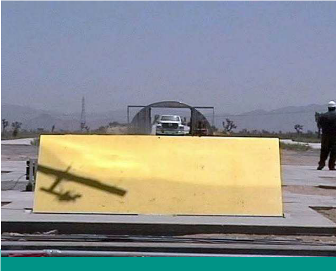
We are testing for your safety. A lorry (15.000 lbs) drives with a speed of 50 mph against the barrier.
