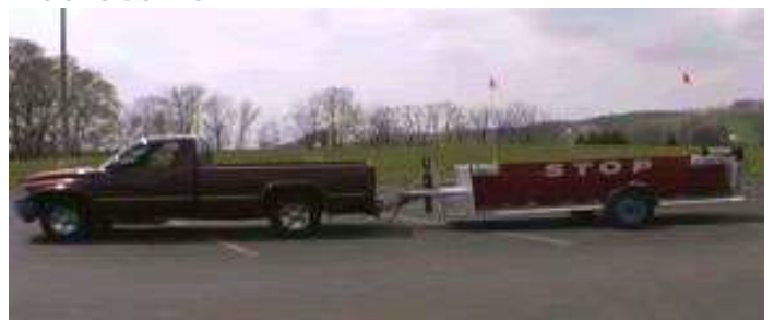
Mobile barrier with removable axle for easy transport.
