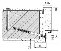
Wall anchor, dowelled with slide anchors (masonry/concrete)
