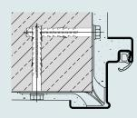
Weld installation with sliding anchor (exposed masonry)
