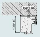
On-site screwmounting and optional factory infill
