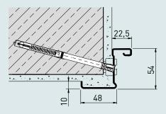
Wall anchor, dowelled, (masonry/concrete)
