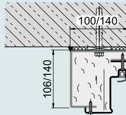
On-site screw-mounting and optional factory infill
