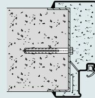
Countersunk screw attachment (lightweight construction stud wall)
