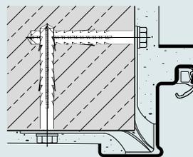
Wall anchor, mortared, (masonry/concrete)
