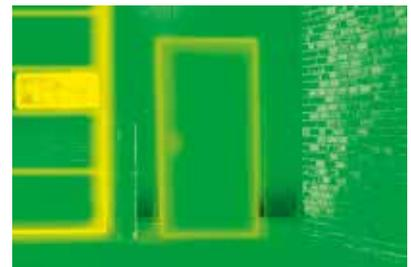
Far smaller energy loss thanks to thermally separated door
