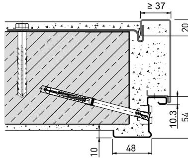
Wall plug and hinged anchor installation (masonry/concrete)
