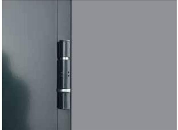
**Construction hinge:** Construction hinges with ball bearings guarantee that opening and closing the door will always be easy. The hinges are integrated in the door leaf and thus have no influence on the visual appearance of the door leaf surface. The door height can be subsequently adjusted with the supplied hinge hook rings up to 4 mm.
