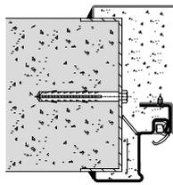
Countersunk screw fastening (lightweight partition)
