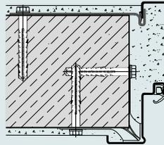
Wall plug and hinged anchor installation (masonry/concrete)
