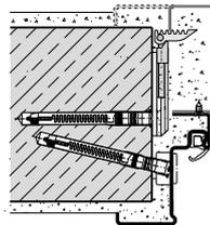
Wall anchor, dowelled with slide anchors
