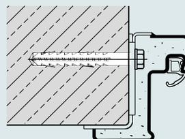
Wall plug installation (aerated concrete)
