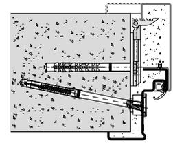
Concealed installation of the counter frame with special fold anchor
