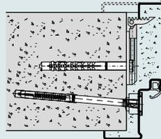
Weld installation with anchor bracket (autoclaved aerated concrete walls)
