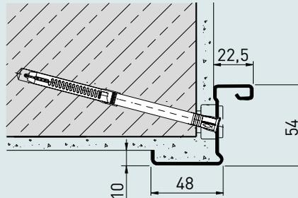
Wall anchor, dowelled, (masonry/concrete)
