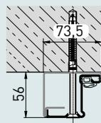
Type 5.3 / 5.3 L Wall plug assembly in the opening (masonry/concrete/steel beams)
