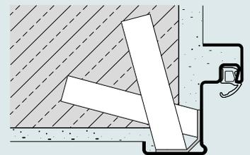
Weld installation with sliding anchor (exposed masonry)
