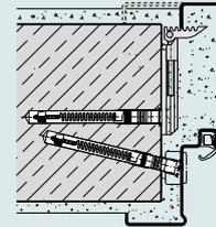
Wall plug and hinged anchor installation (exposed masonry/autoclaved aerated concrete walls)
