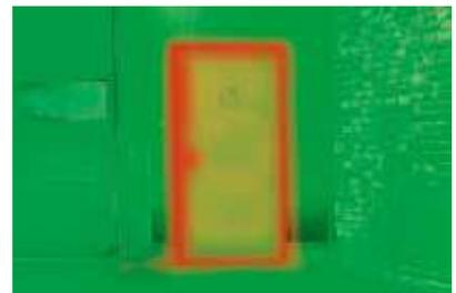
Visible energy loss without thermally separated door
