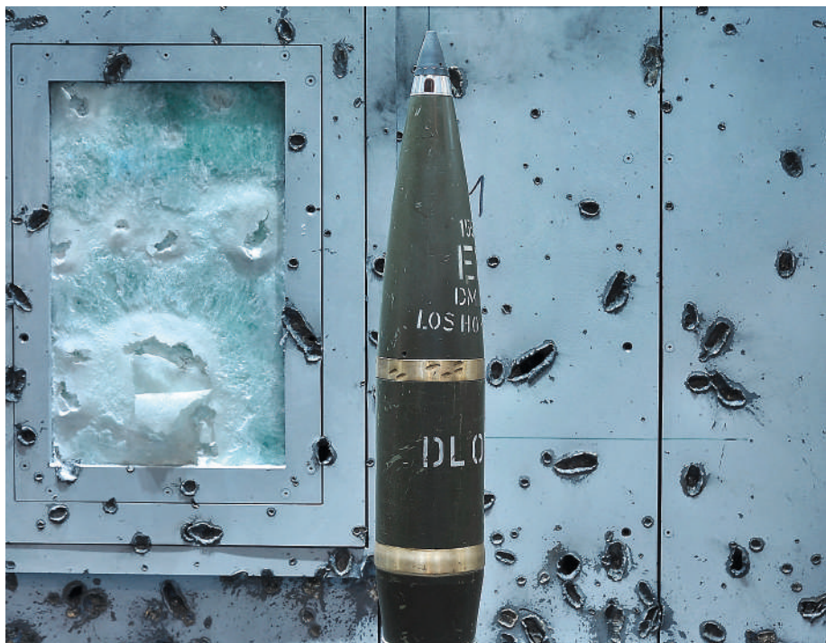
The construction successfully passed the test with artillery shells (155 mm, approx. 43 kg) that were detonated at a distance of 1.5 m from the unit.
